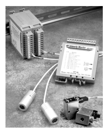
The user also has the use of two relay circuit connections. If the UV lamp's intensity goes below a set intensity, these outputs will switch in an indicating circuit of the user's design.
